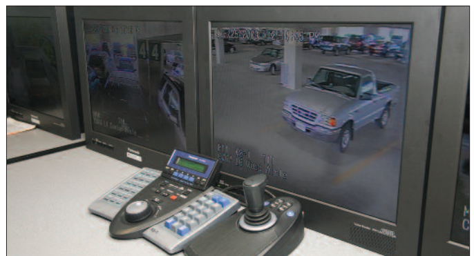
The Panasonic WV-CU650 system controller provides a jog dial and shuttle ring for smoother system control, and a detached joystick allows operators to pan, tilt and zoom easily.
